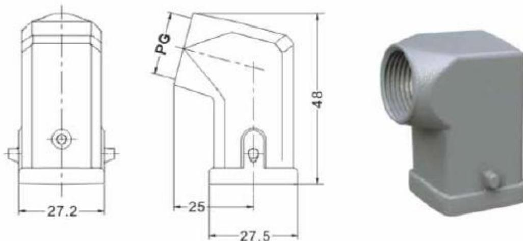
**Plug to be fixed on the extension cable: CMB\_04\_Px\_D\_R\_010**
